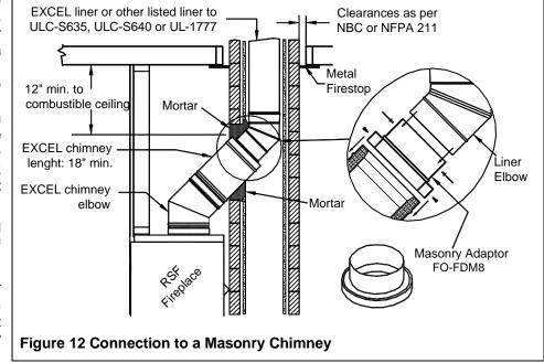
If it is difficult to install rigid stainless steel liner in the existing masonry chimney or for a masonry chimney with less than 10"x10" inside, a listed stainless steel flexible liner can be used along with a flexible/rigid adaptor (LM-8LAF) available from your RSF dealer.
