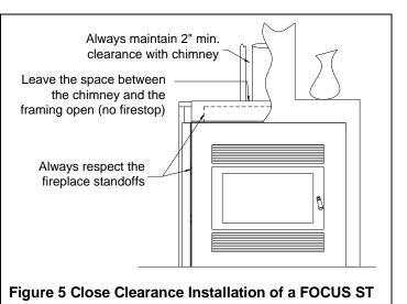
Under no circumstances should the distance between the ceiling firestop and the base fireplace be less than the dimension specified in Table 1 (C).
