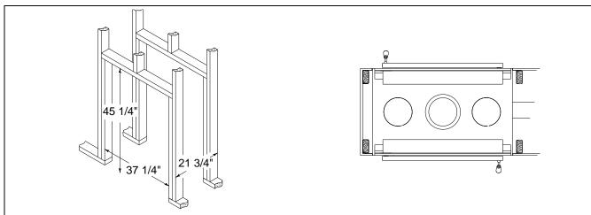
The framing dimensions are larger than required for ease of installation.
